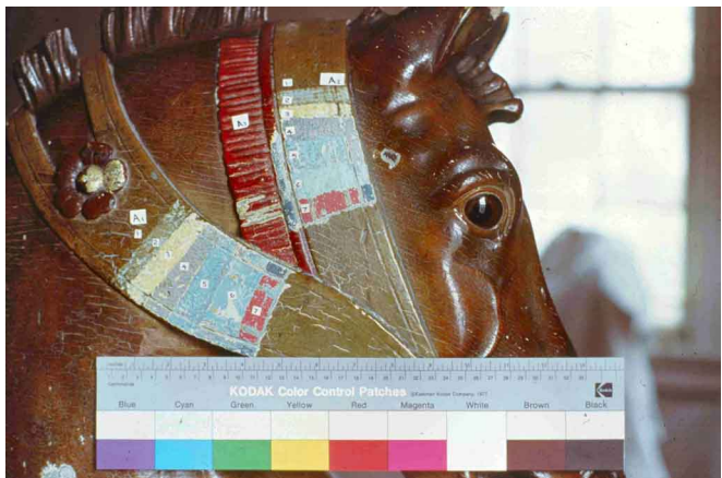
The samples on the bridle show each layer of paint.
